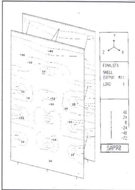
Fig 3: Finite Element Analysis model. The specimens modeled a typical section one bale long, but without actual straw, as the straw would conceal important events occurring within the specimens during testing. However, the tests showed that the presence of the straw bales would improve the performance of the walls, and subsequent tests should include the material.
